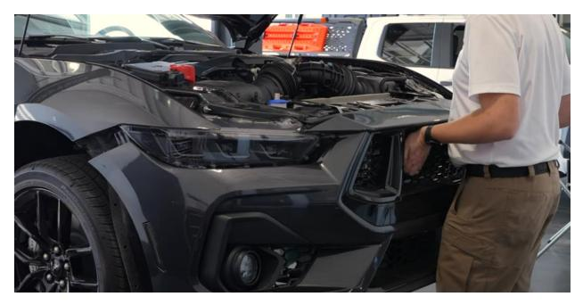
Hang the bumper assembly back onto the vehicle, ensuring it is properly seated on the hangers.
