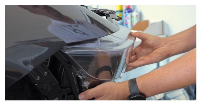
Partially remove the passenger-side headlight using **13mm and 10mm sockets** to remove two screws and one nut.
