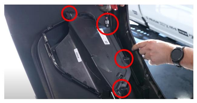
If your vehicle is equipped with corner grille backer plates, remove them using a **7mm socket**. For vehicles with an air duct on the driver's side, remove it in the same fashion.
