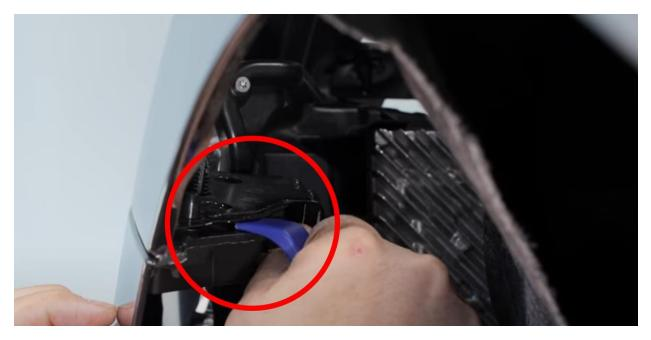
Detach the bumper from the corner panel using a trim removal tool. **Repeat this process** for both sides.
