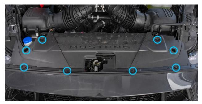
Start by removing the **engine cover** to access the fasteners below. Use a **trim removal tool** to remove **eight push pins**, then set the cover aside.
