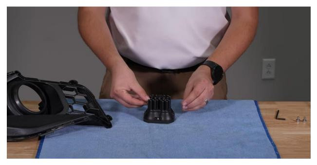
For **SS3 Pods**, assemble the pods by placing the locking nuts with nylon rings facing inward.
