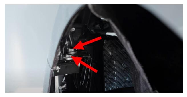
Use a 10mm wrench to remove the two screws securing the bumper to the corner panel.
