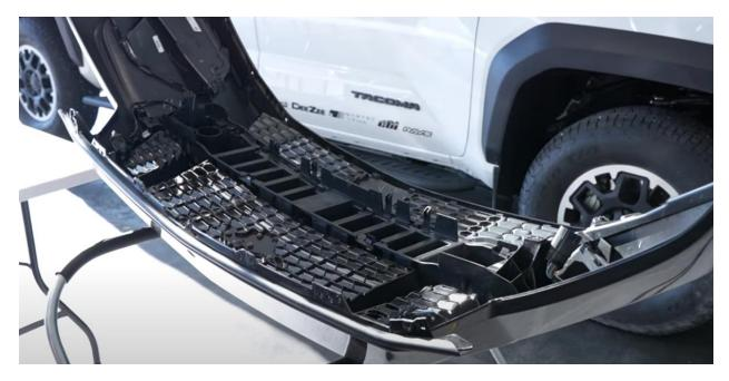
Carefully lift the bumper assembly off the five hangers at the top and pull it away from the vehicle. Place the bumper on a cradle or soft surface.
