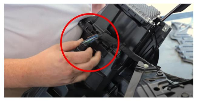
Pull the headlight out and disconnect the **multi-pin connector** on the back.
