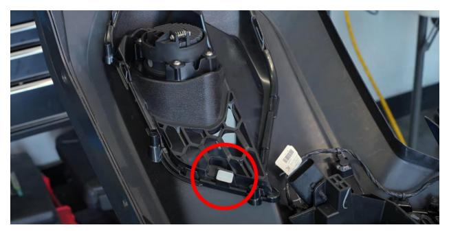
Reinsert the white safety pin to lock it in place. Repeat this process for the other side.
