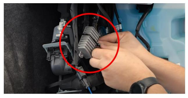
Secure the **solid-state relay** away from hot or moving parts using zip ties or 3M tape.
