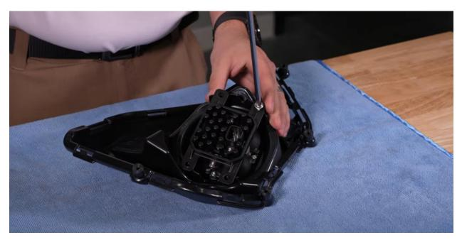
Use a **Phillips head screwdriver** to secure the pod to the bezel with the included screws.
