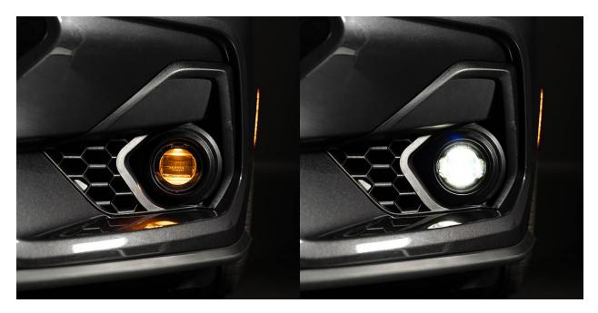
Test the fog lights to ensure proper functionality. The amber backlight should activate with the parking lights, and the main beam should turn on with the low beams.
