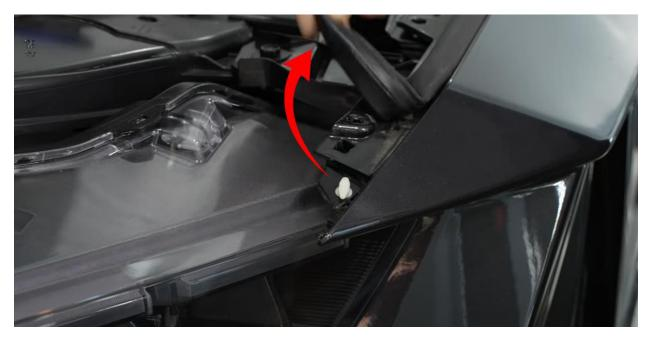
Partially detach the weather stripping from the T-clip near each headlight to gain better access.
