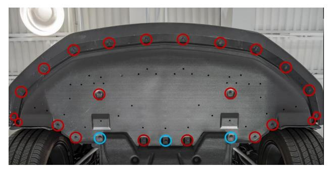
Underneath the vehicle, use a **7mm socket** to remove **22 screws** securing the lower bumper. Use a **trim removal tool** to remove **three push pins**, then slide the shield rearward to release it.
