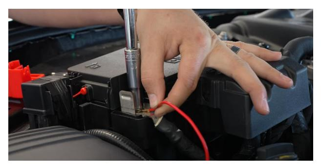
In the engine bay, use **8mm and 10mm sockets** to loosen the battery terminals. Connect the positive and negative leads from the fog light harness to the battery.
