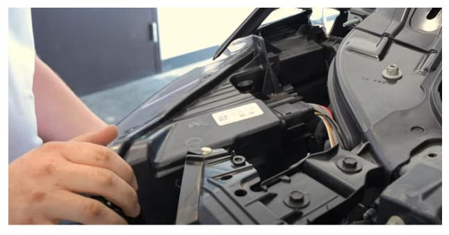
Let the remaining harness hang down, and reinstall the headlight.
