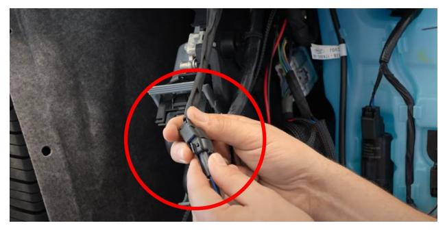
Plug the fog light harness into the factory side marker harness.
