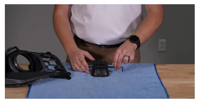
Slide the **Type A bracket** over the pod and secure it with **5/32-inch Allen screws** and washers.
