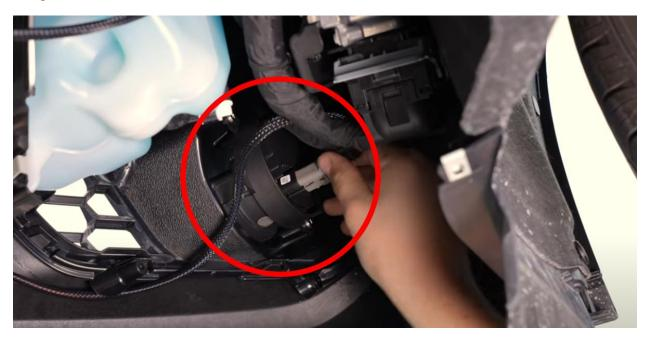
Reconnect the side markers, multi-pin connectors, and DT output leads to the fog lights.
