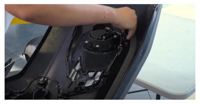
Install the assembled fog light bezels into the bumper. Ensure all plastic tabs are aligned, and press firmly to seat the bezel.
