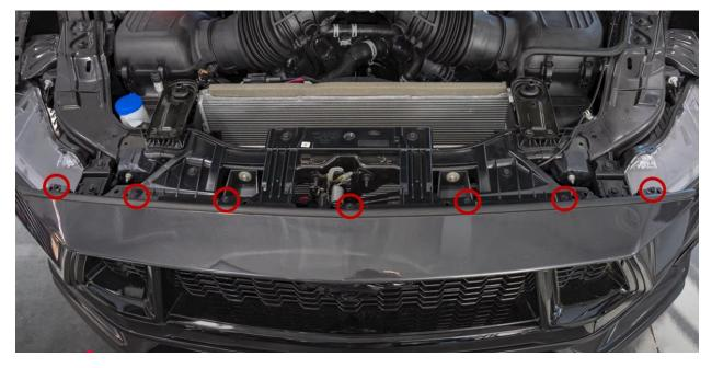
Step 2 - Remove the Top Bumper Screws
