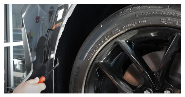
Move to the wheel wells and use a **trim removal tool** to remove **five push pins** on each side. Push the fender liner back to access the fasteners.
