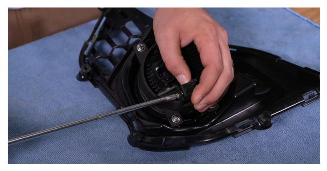
For **Elite Series Lamps**, secure the lamps with the included screws, then use the aiming tool to adjust the lamps before installation. Repeat these steps for both sides.
