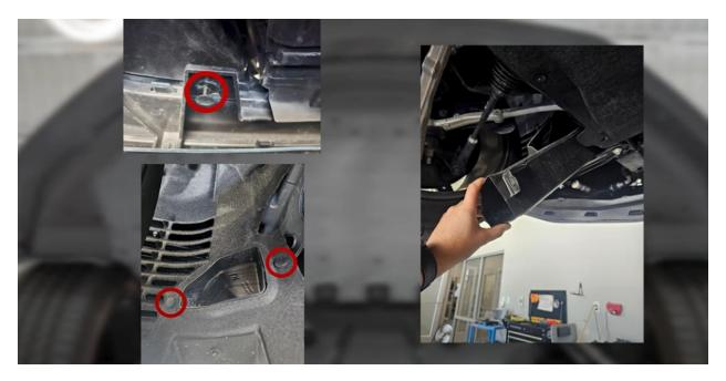
If your Mustang is equipped with brake ducts, remove the **three push pins** on both the driver and passenger sides, then slide the brake ducts rearward to remove them.
