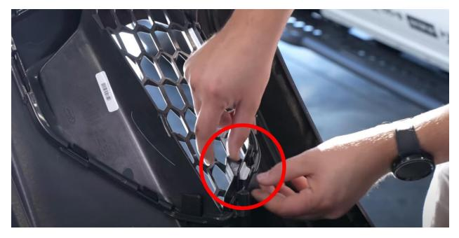
Release the corner grilles by depressing the white safety pins, applying outward pressure on each clip, and removing the grilles. Repeat this for both sides.
